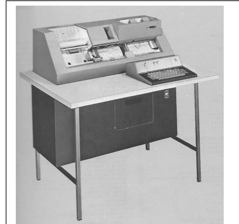
The IBM 029 punch machine by which we transferred FORTRAN code and data onto punch cards. (From IBM Reference Manual, IBM 29 Card Punch, eighth edition, 1971. )
